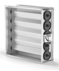
Multi-plane dampers control or close airflow in ventilation ducts. The multi-plane damper consists of a housing made of galvanized profiles and aluminum blades. The blade height is the same for dampers of all sizes. This damper is controlled by means of a manual mechanism. The mechanism consists of a short axle, a long axle and toothed gears outside the damper, mounted on
