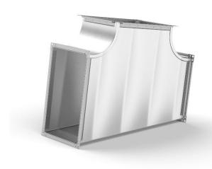
Tapered three-ways are terminated with frames made of profiles and are additionally reinforced with transverse sheet corrugation. The tapered three-way features a branch at an angle of 90° and reduction of the main duct.
