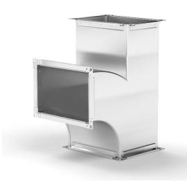
Three-ways with take-off bend are terminated with frames made of profiles and are additionally reinforced with transverse sheet corrugation. The take-off bend allows for a smooth air distribution without increasing turbulence.
