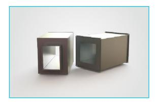
Preinsulated elements are rectangular ducts and fittings having mineral wool insulation. The system ensures reduction of heat loss, tightness of elements and their connections, and suppression of noise generated by air flowing inside the ventilation line. Preinsulated elements come in two types made of stainless steel grade AISI 304 and stainless steel with increased corrosion resistance grade AISI 316.
